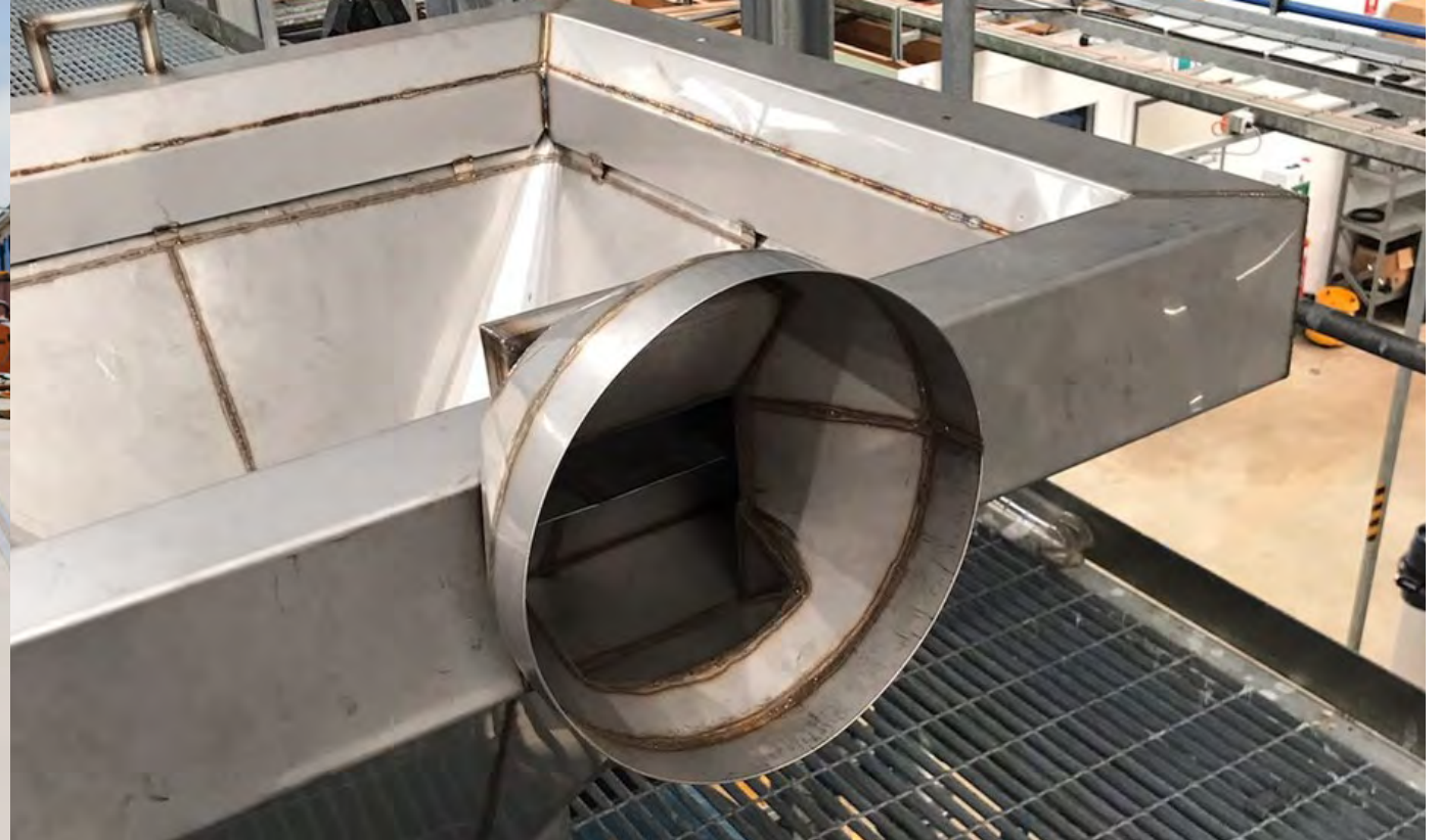
The vacuum funnel for powdered chemicals reduces dust and chemicals in the work environment
