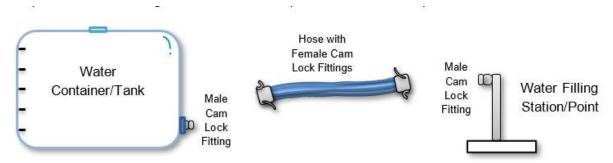
When filling up from the container's cam lock, open the cap on the top of the container.
