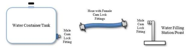
When filling up from the container's cam lock, open the cap on the top of the container.
