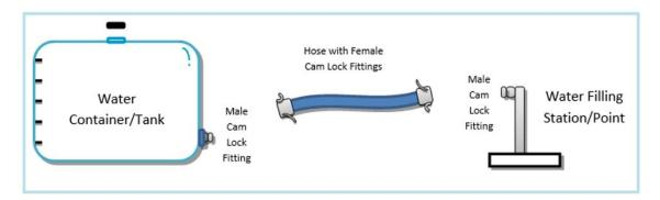
The picture above provides an example of the hose fittings and connections required for a safe fill of your container/tank. When filling from a water filling station, we insist that you connect your hose fitting to the cam lock connection at the filling point with the cam lock connection on your water tank.
