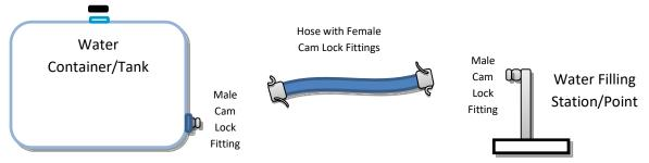
When filling up from the container's cam lock, open the cap on the top of the container.
